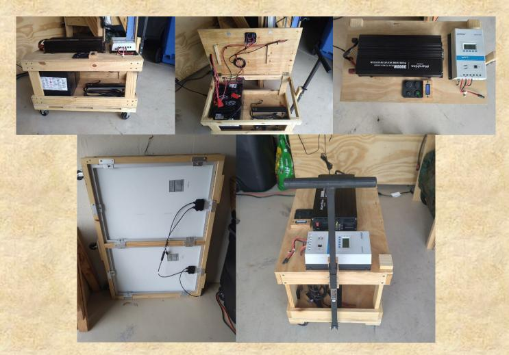
**System Basics:** 3000W/6000W peak Pure Sine Wave Inverter | 4 x 100W, HQST Solar Panels EPEVER MPPT Solar Charge Controller | 2 x 6V/230AH Deep Cycle Golf Cart Batteries
